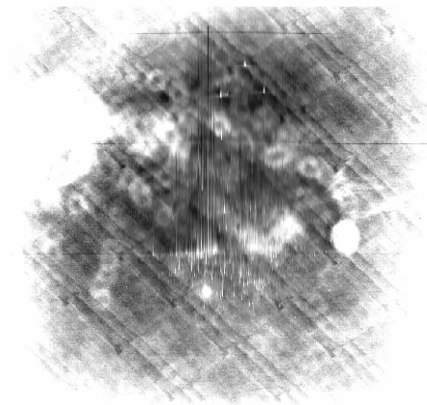
Fig. 7 A dome flat frame where the blooming occurs before full-well
