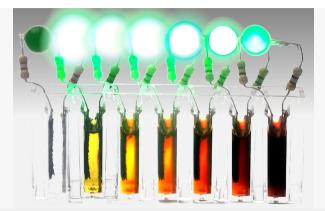
Time-lapse series of images shows the new type of battery becoming fully discharged over a period of days. In the process of discharging, the new "catholyte" material in the battery cell gets chemically coverted into a reddish compound, so the color gets darker the more it discharges.
