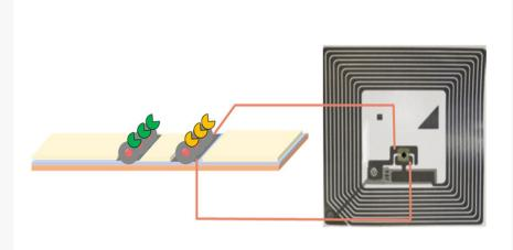
In this lateral flow assay, the paper that wicks the solution (left) has control and test lines that can be wired in parallel with the integrated circuit of an RFID device for wireless detection by a smartphone.
