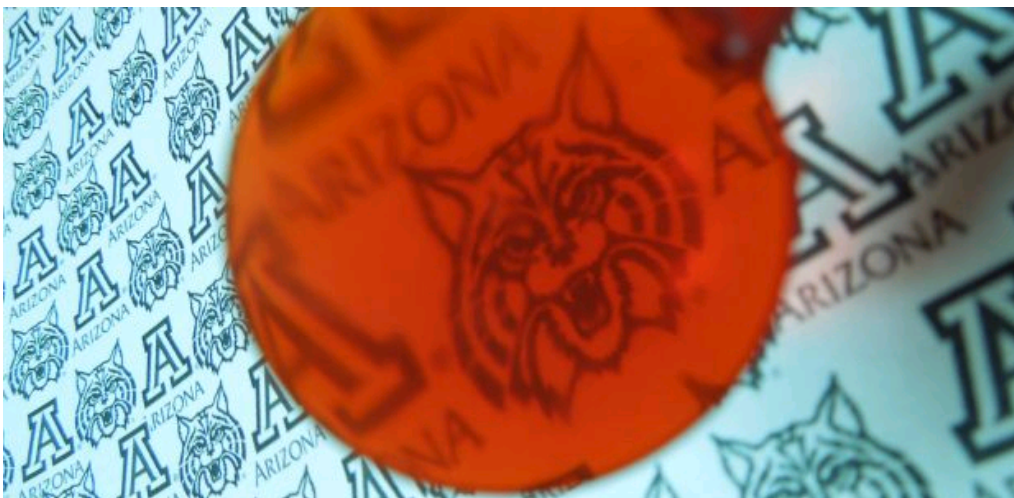
A UA-ed research team has discovered a simple process for making a new lightweight plastic from the inexpensive and abundant element sulfur. This plastic can be made into easy-to-make, lightweight lenses that transmit infra-red light. Photo credit: Jared Griebel/ Pyun lab, University of Arizona department of chemistry and biochemistry.
