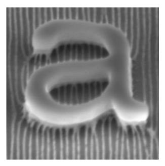
Cross-section scanning electron microscopy image after hydrogen silsesquioxane patterning, sequential infiltration synthesis and removal of initiated chemical vapor deposition topcoat and organic components. (Image by Hyo Seon Suh / University of Chicago)
