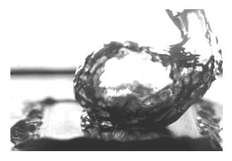
High-speed video of the researchers' test setup shows water boiling on a specially treated surface, which causes bubbles to form at specific separate points rather than spreading out in a film across the surface, thus leading to more efficient boiling. The video has been slowed down by 100 times to show more detail.
