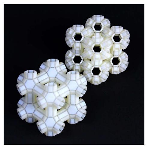
Harvard researchers have developed a general framework to design reconfigurable metamaterials that is scale independent, meaning it can be applied to everything from meter-scale architectures to reconfigurable nano-scale systems (Image courtesy of Johannes Overvelde/Harvard SEAS).
