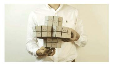
The same computational models can also be used to quantify all the different ways in which the material could bend and how that affected effective material properties like stiffness. This way they could quickly scan close to a million different designs, and select those with the preferred response.
