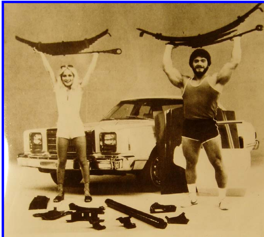
Figure 8-34 Experimental composite car. A weight comparison; a graphite truck spring (left) versus steel spring (right). (Ford Motor Co.)
