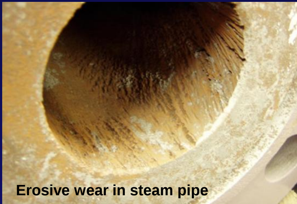
(a) 蒸汽管冲蚀形态
