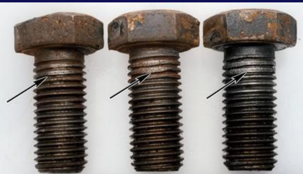
(a) 螺栓的微动磨损
