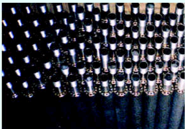
Fig.2 Titanium anode pipes with nanostructured
