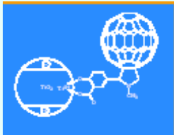
A self-assembled monolayer of SFP onto TiO2 nanocrystalline
