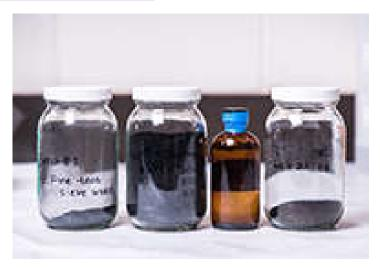
These jars show variations of a Kansas State University-patented liquid polymer that looks like water and has the same density and viscosity as water. The polymer becomes a ceramic when heated and can be mass-produced.
