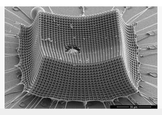
Engineers at MIT, Caltech, and ETH Zürich find "nanoarchitected" materials designed from precisely patterned nanoscale structures (pictured) may be a promising route to lightweight armor, protective coatings, blast shields, and other impact-resistant materials.
