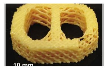
Graphic showing a concept device of a spinal cage with a porous lattice architecture. Credit and Larger Version (/discoveries/disc\_images.jsp?cntn\_id=300754&org=NSF)
