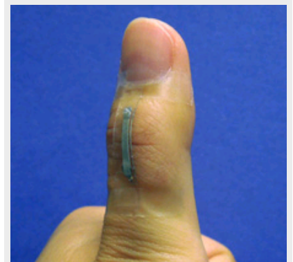
A sensor based on silver nanowires is mounted onto a thumb joint to monitor the skin strain associated with thumb flexing. The sensor shows good wearability and large-strain sensing capability. Click to enlarge. (Photo: Shanshan Yao.)
