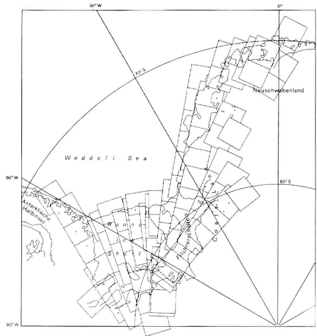
Fig. 4 - Imagery coverage diagram of Landsat MSS mosaic "Filchner-Ronne-Schelfeis, Coats Land and Neuschwabenland". Indicates geodetic control by GPS or Doppler satellite positioning used for the southern part (After: Sievers et al. 1989, Heidrich et al. 1991).
