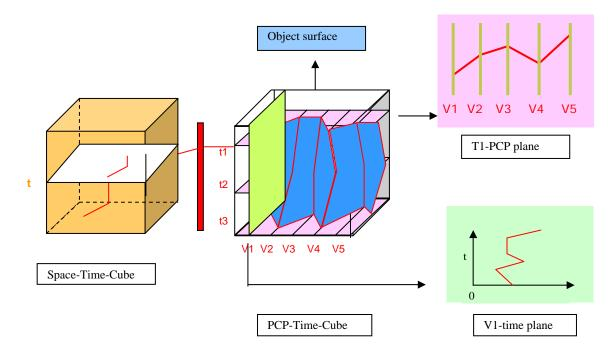
Figure 3. The Parallel-coordinate-plot Time Cube Model (PTC). On the left a STC link to PCP-Time-Cube and on the right the views are vertical plane and horizontal plane from the PTC.
