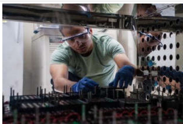
Rice University graduate student Sebastián Castillo-Hair conducts tests with the Light Plate Apparatus, an open-source optogenetics research platform developed in the laboratory of Rice's Jeffrey Tabor, assistant professor of bioengineering. (Photo by Jeff Fitlow/Rice University)
