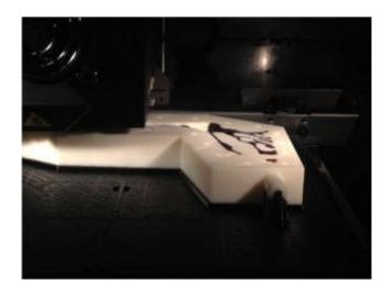
Partially completed 3D printed model of nostril to trachea airway showing fine structure of the nasal cavity.
