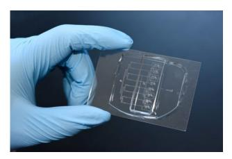
Researchers, led by Sindy Tang, assistant professor of mechanical engineering at Stanford, have created a new tool for cutting cells, called a microfluidic guillotine. This eight-channel version of their tool can cut cells over 200 times faster than conventional methods. (Image credit: L.A. Cicero)
