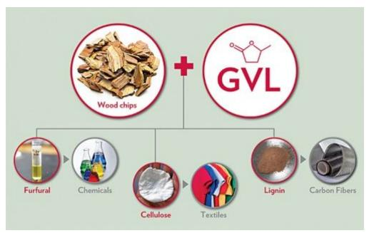
UW-Madison researchers and collaborators have developed a new "green" technology for converting non-edible biomass into three high-value chemicals that are the basis for products traditionally made from petroleum. GRAPHIC COURTESY UW-MADISON/PHIL BIEBL
