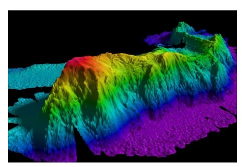
A map of a seamount in the Arctic Ocean created by gathering data with a multibeam echo sounder, Researchers have found that such topographic features can trap deep waters and produce turbulence.
