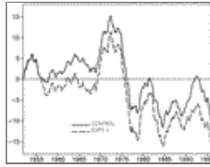
Fig. 2. Influence of bias on analysis. Sea level from control analysis ( \alpha = 0 ) and expt 1 ( \alpha = 0.7 ) in the central North Pacific ( 49^\circ N, 184^\circ W). The average difference is 3.9 cm.
