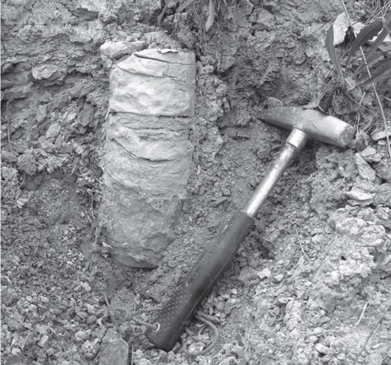
Figure 3. Vertical fluid conduit cemented by CH_4 -derived dolomite occurring within lower Messinian marls.
