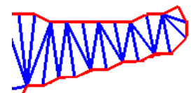
Figure 2b. Blue triangle edges are filtered out as they are bounded by the same spectral edge (in red).
