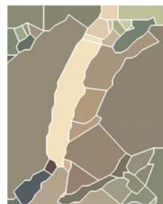
Figure 1d. Result of vectorizing image 1a. Polygons (white boundaries) built by grouping triangles.
