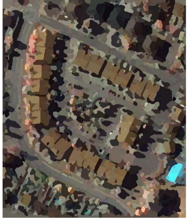
Figure 5b. Result of vectorizing image 5(a). Fine, 0 th , level of detail: 2,612 polygons.
