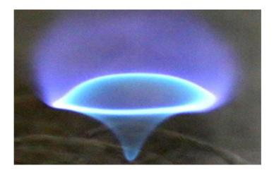
Researchers have identified the structure of a "blue whirl," an avenue for low-emission combustion. <u>Credit and Larger Version (/discoveries/disc\_images.jsp?cntn\_id=301658&org=NSF)</u>
