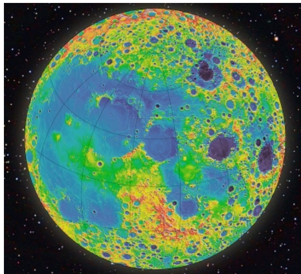
Using measurements taken by an instrument onboard NASA's Lunar Reconnaissance Orbiter spacecraft, researchers have mapped all large craters on the moon. In this image, blue indicates low elevation, and red indicates high elevation. Image: NASA/LRO/LOLA/GSFC/MIT/Brown
