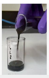
MIT researchers have developed a novel semisolid flow battery that uses a mixture containing dispersed manganese dioxide particles, along with an electrically conductive additive called carbon black, that enables efficient electrochemical energy conversion when reacted with a zinc suspension or plate.
