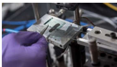
Water-based electrochromic film blade coating
