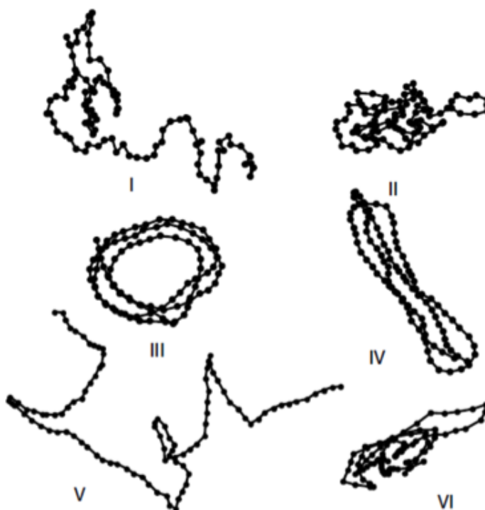
Figure 2.4: Typical conformations of a 100-segment PPV homopolymer generated by Monte Carlo simulations. See Hu et al 41 (permission license number 3401051508068).
