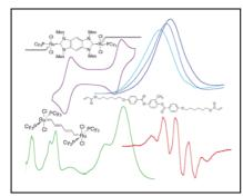
The collage at right represents several of the methods and molecules used by our group. Clockwise from upper left, the methods are cyclic voltammetry (showing reversible transformations among three oxidation levels), IR spectroscopy (expanded spectra of three different redox levels), EPR spectroscopy (used to characterize mixed-valence states), and UV-Vis-Near IR spectroscopy (showing a variety of electronic
