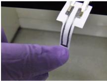
The students then turned to the traces of a bendable toy pencil. (These novelty pencils are flexible because the graphite is mixed not with clay, but with a polymer binder.) Again, conductivity could be increased and decreased by manipulating the paper, but the students found it also was affected by the presence of volatile chemical vapors, such as those from toxic industrial solvents.
