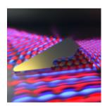
New zero-index material made of silicon pillar arrays embedded in a polymer matrix and clad in gold film creates a constant phase of light, which stretches out in infinitely long wavelengths. (Illustration by Credit: Peter Allen/Harvard SEAS)
