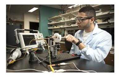
Researcher Federico Hita fine-tunes a hand-cranked piezoelectric device developed to generate plasma <u>Credit and Larger Version (/discoveries/disc\_images.jsp?cntn\_id=301170&org=NSF)</u>
