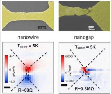
Rice University scientists discovered that "hot" electrons can create a photovoltage about a thousand times larger than ordinary temperature differences in nanoscale gaps in gold wires. On the left, a laser-heated, bowtie-shaped plasmonic gold nanowire created a small voltage in the wire. On the right, a gold nanowire with a nanogap under the same light source showed a much stronger voltage at the break. Click on the image for a larger version. Courtesy of the Natelson Group
