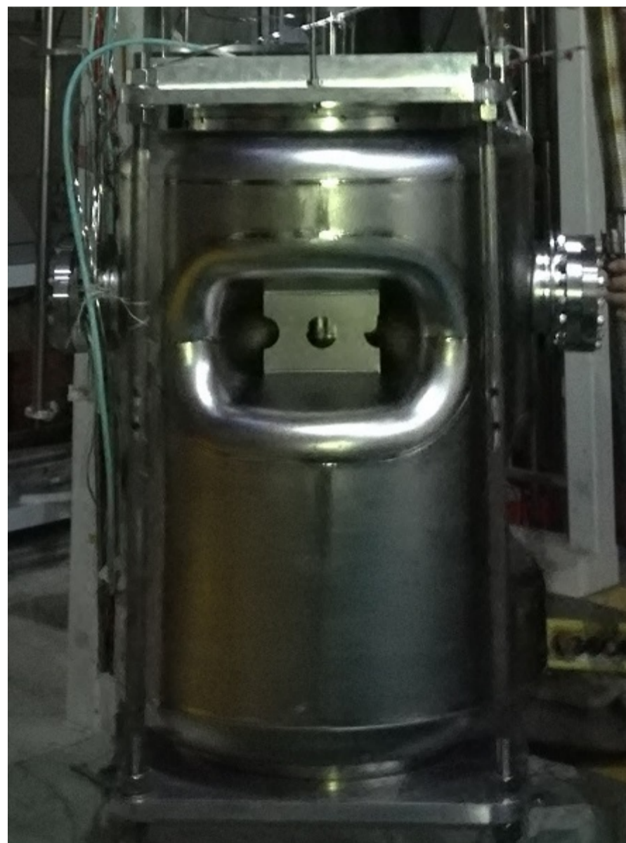
即将进入杜瓦进行垂测的双Spoke腔
