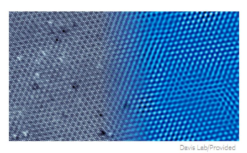
This composite image shows where the selenium atoms reside in the crystal of niobium diselenide, a transition metal dichalcogenide, using conventional scanned tunneling microscopy (left, in grey) and where the electron pairs are observed using scanned Josephson tunneling microscopy (right, in blue).
