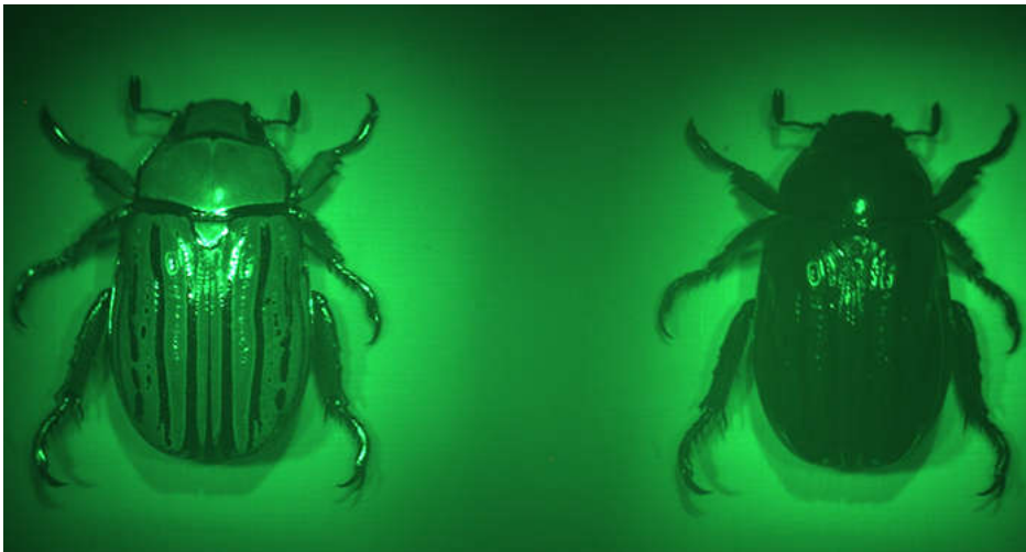
Imaging with the multispectral chiral lens forms two images of the beetle, Chrysina gloriosa , on the color camera (Image courtesy of the Capasso Lab/Harvard SEAS)
