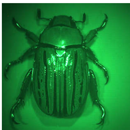
An image of a beetle taken by a multispectral chiral metalens is formed by focusing left-circularly polarized light reflected from the beetle (Image courtesy of the Capasso Lab/Harvard SEAS)
