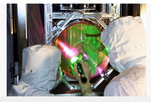
MIT scientists have cooled a 10-kilogram object to a near standstill, using LIGO's precise measurements of its 40-kilogram mirrors. Shown here are LIGO optics technicians examining one of LIGO's mirrors.
