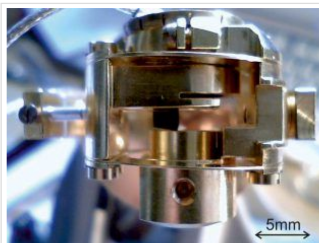
Physicists at Karlsruhe Institute of Technology used this capacitive dilatometer to measure the thermal expansion in cerium copper gold alloys cooled to temperatures very close to absolute zero with a precision of one tenth of a trillionth of a meter, or approximately one-thousandth the radius of single atom. The precise thermal expansion measurements allowed the researchers to map out the stress dependence of entropy in materials as they were cooled to the point of a quantum phase transition. (Image courtesy of K. Grube/Karlsruhe Institute of Technology)
