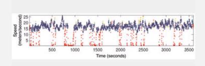
IODA separated good and bad data from an anemometer: blue=high-quality; red=low-quality. Credit and Larger Version
